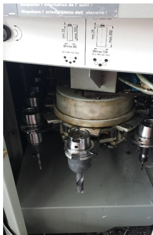
Cambio utensile 30 posti – ATC 30 positions – Entrepot d'outils a30 positions – 30 position Werkzeugwechsler
